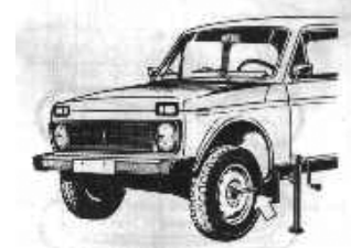
Fig 53. Jacking up car for replacement of wheels.
